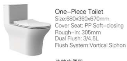
One-Piece Toilet Size:680x360x670mm Cover Seat: PP Soft-closing Rough-in: 305mm Dual Flush: 3/4.5L Flush System:Vortical Siphon 連體座便器 尺寸: 680x360x670mm 蓋板: PP緩降蓋板 坑距: 305mm 名義用水量: 3/4.5L 沖水系統:旋渦虹吸
