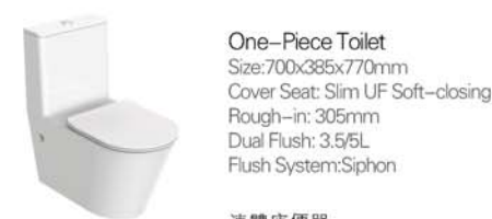
One-Piece Toilet Size:700x385x770mm Cover Seat: Slim UF Soft-closing Rough-in: 305mm Dual Flush: 3.5/5L Flush System:Siphon 連體座便器 尺寸: 700x385x770mm 蓋板: UF緩降薄蓋板 坑距: 305mm 名義用水量: 3.5/5L 沖水系統:虹吸
