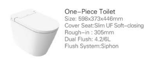
One-Piece Toilet Size: 598x373x446mm Cover Seat: Slim UF Soft-closing Rough-in : 305mm Dual Flush: 4.2/6L Flush System:Siphon 一體座便器 尺寸: 598x373x446mm 蓋板: UF緩降薄蓋板 坑距: 305mm 名義用水量: 4.2/6L 沖水系統:虹吸
